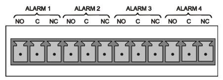
Figure 3-13: Concentration Alarm Relay
